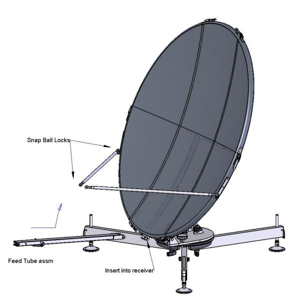
3. Attach each side strut. Snap on to side panels first then snap to corresponding ball snap on the Feed Tube assembly.
